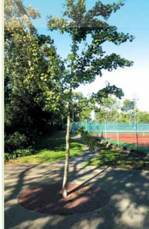
'Surface materials around trees in hard landscapes' are the subject of an LTOA working party. This shows a recently planted Ginkgo biloba tree with a neat circular surround of 'bonded gravel'.
